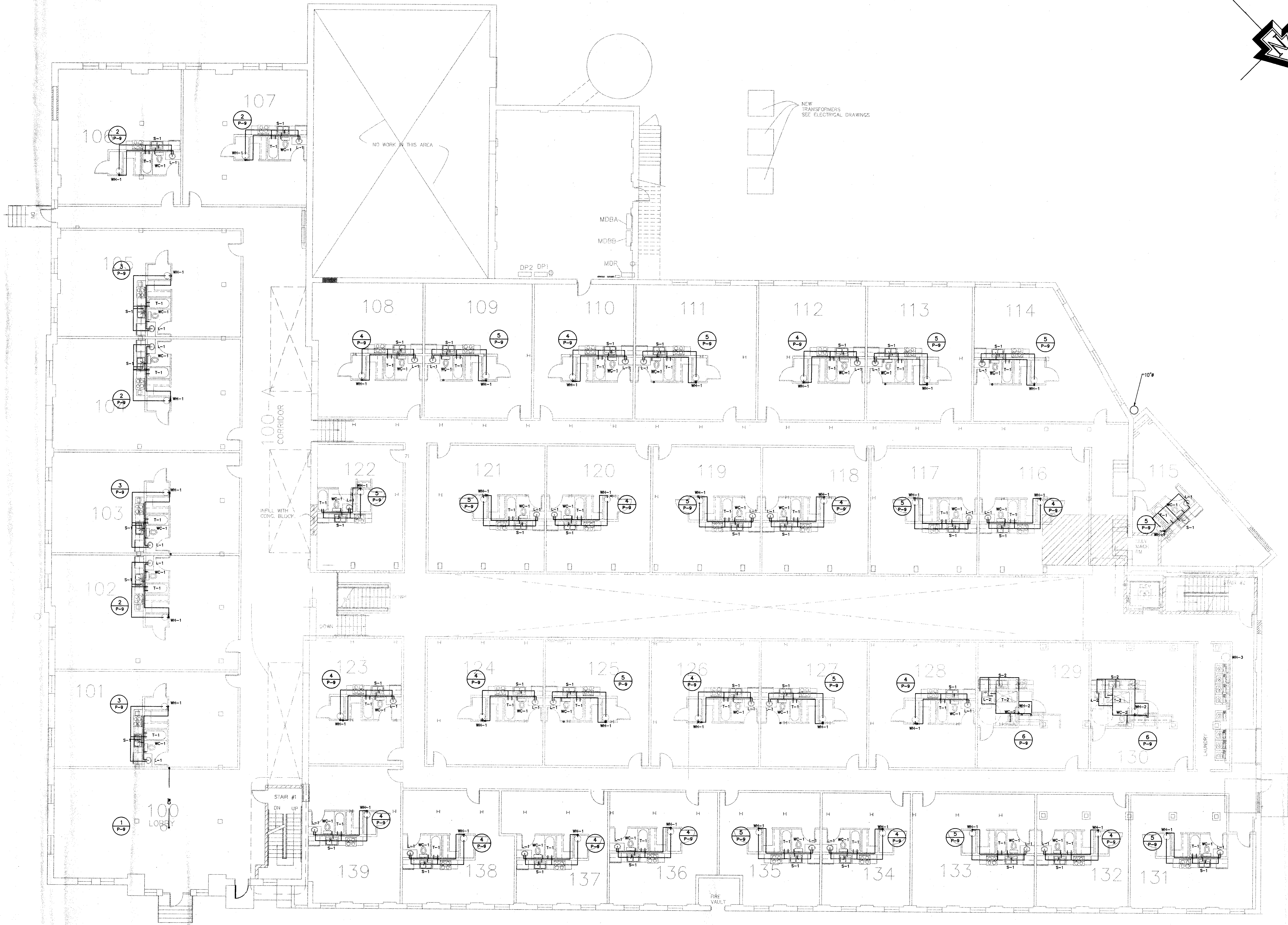
FIRST FLOOR POTABLE WATER PLAN, TYPICAL FOR SECOND & THIRD LEVELS WHERE APPLICABLE
