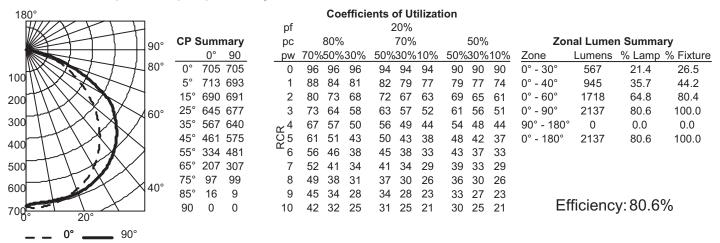
\*The LER (Luminaire Efficacy Rating) is the lumens per watt rating for this fixture. It is used to compare the energy efficiency of various products. This photometric report is based upon IES testing procedures, as stated in LM-41-1998.
