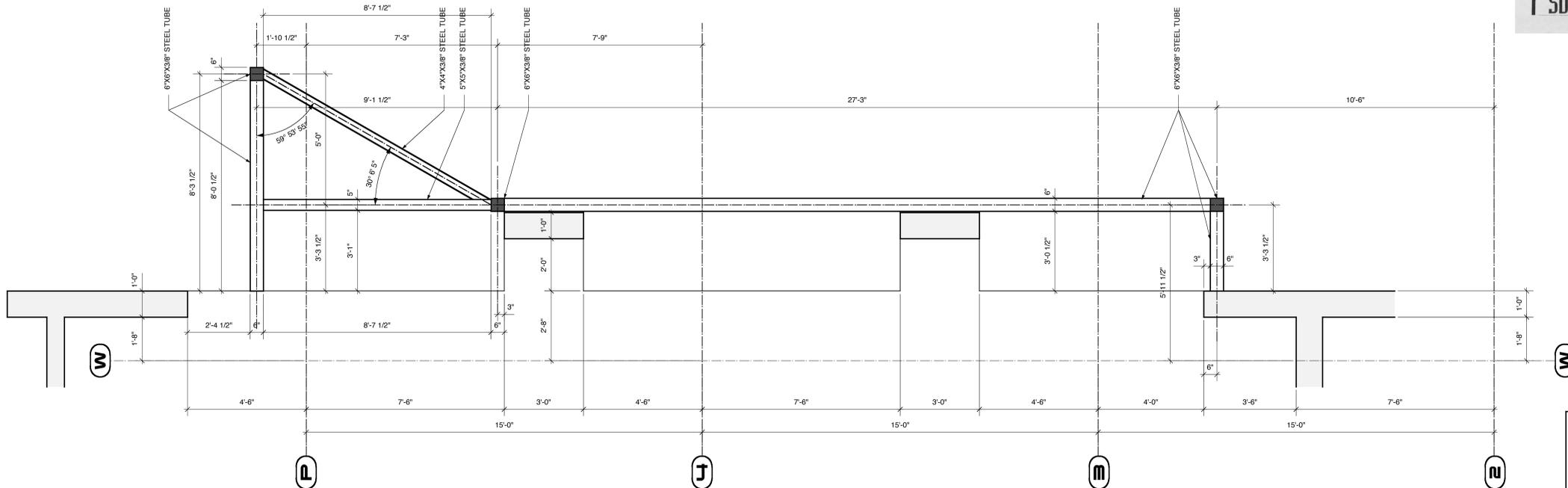
**SD-041** STRUCTURAL STEEL FRAME @ STAIR B
