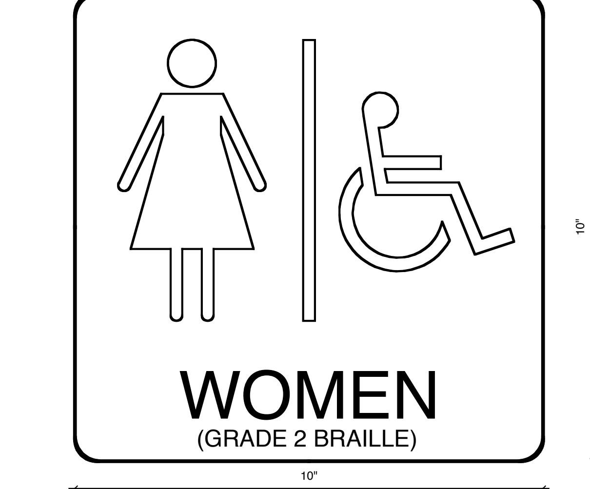
6 TYPICAL ELEVATION @ SIGN 6" = 1'-0"
